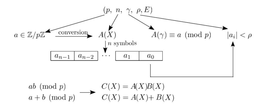
$E \in \mathbb{Z}[X]$  a monic polynomial with deg(E) = n and  $E(\gamma) \equiv 0 \pmod{p}$ , used for External Reduction.
